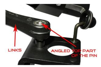
4. ATTENTION! Make sure the pin goes all the way through the links. The angled top part of the pin must come out above the links, like in the picture below. If this is not done correctly, the bearings might break.
