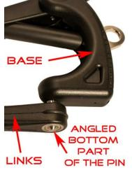
6. ATTENTION! Make sure the pin goes all the way through the links. The angled bottom part of the pin must come out underneath the links, like in the picture below. If this is not done correctly, the bearings might break.
